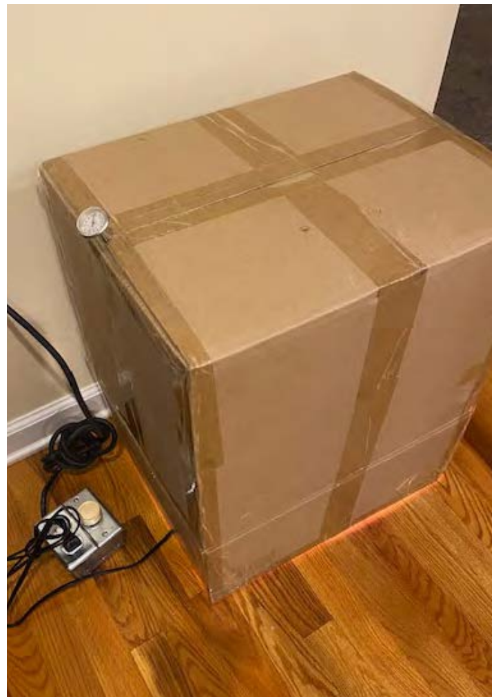
A dimmer switch allows Dave to regulate the put out by the 100-watt bulb, and a meat thermometer helps him monitor the temperature inside the warming chamber.
