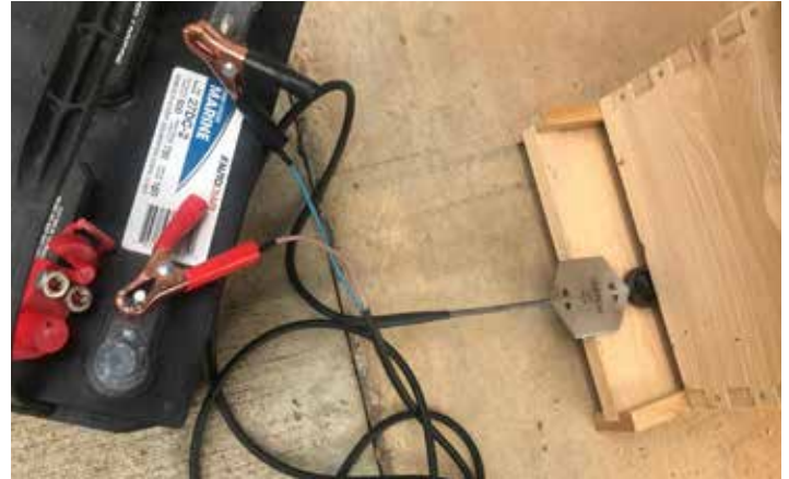
(Figure 2) Oxalic Acid vaporized by attaching to a battery.
