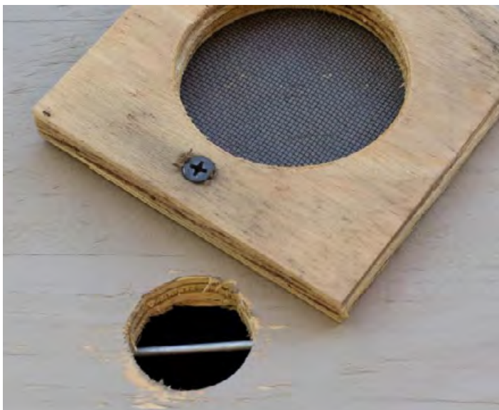
An entrance gate can be added for transporting the bees. The entrance gate was created by drilling a 2" hole in the center of a 4" x 4" chunk of plywood, and then covering one side with screen.
